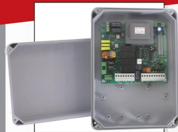
**CB2 - CONTROL BOARD FOR 1-2 OPERATORS 230V – WITH RX 433.92 ON BOARD SOFT STOP / PEDESTRIAN**
