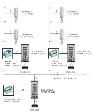
System MATIBUS enables creation of multi-entrance structure, with distribution on:
