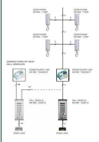
MATIBUS system can be extended up to maximum 8 main call station. Durning a conversation between one station and a user, all remaining stations are occurred. One of call stations must be powered by power supply unit ref. 1052/30P, the rest call stations by power supply units ref. 1042/20P.
